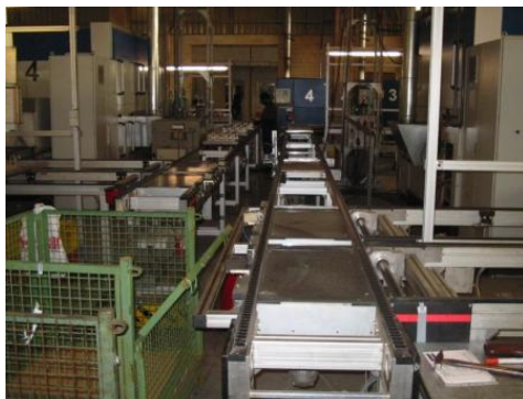
Fig: Examples of the excessively long conveyors necessary to hold production buffer stock which compensates for poor productivity and Laser 3 before the POKe YOKE process monitoring (weld temperature & focal point/focal length) for leading indicators.
