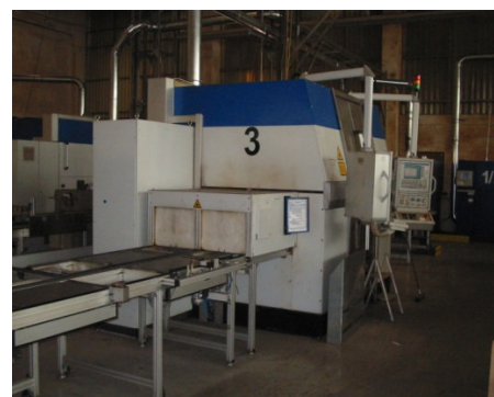
Fig: Examples of the excessively long conveyors necessary to hold production buffer stock which compensates for poor productivity and Laser 3 before the POKe YOKE process monitoring (weld temperature & focal point/focal length) for leading indicators.
